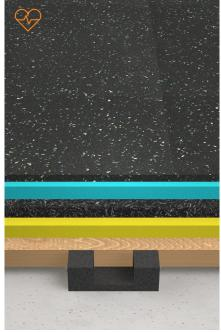
Cardio zones require floor systems to isolate the accumulative low frequency vibration created by multiple treadmill and spinning bike activities. The **ISO-Flex** Cardio systems isolate this vibration, preventing low frequency sound transmitting through the structure.
